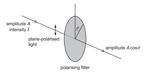
The intensity of the initial beam is I.
